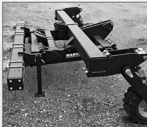
DUAL FRAME 3PT BAR FACILITATES COULTERS IN FRONT & ROW UNITS IN BACK.
