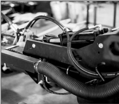
HYDRAFLEX™ CYLINDER OPTION ENABLES 18° UPWARD WING FLEX
